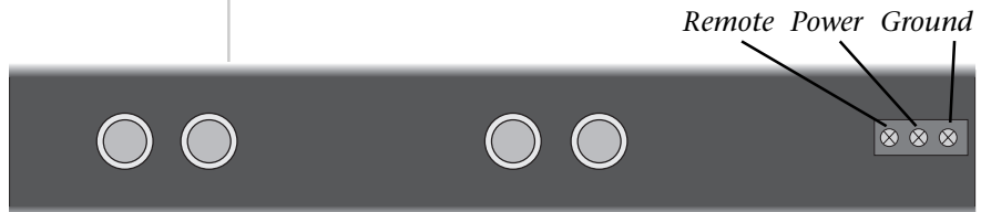
Figure 3: Side view of DQT with power connector and RCAs
