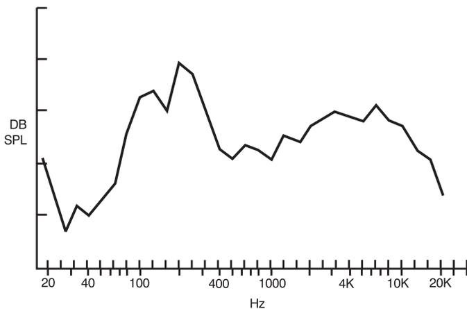
*Fig. 2 The un-equalized 1/3 octave satellite response for an "optimally" placed driver.*
