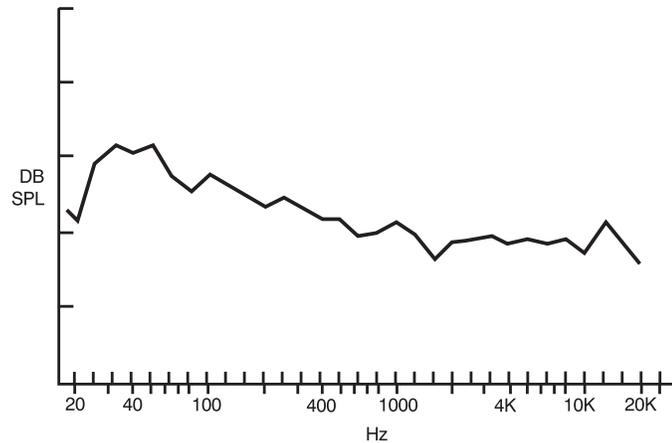
Fig. 4 The total system acoustic 1/3 octave system response.
