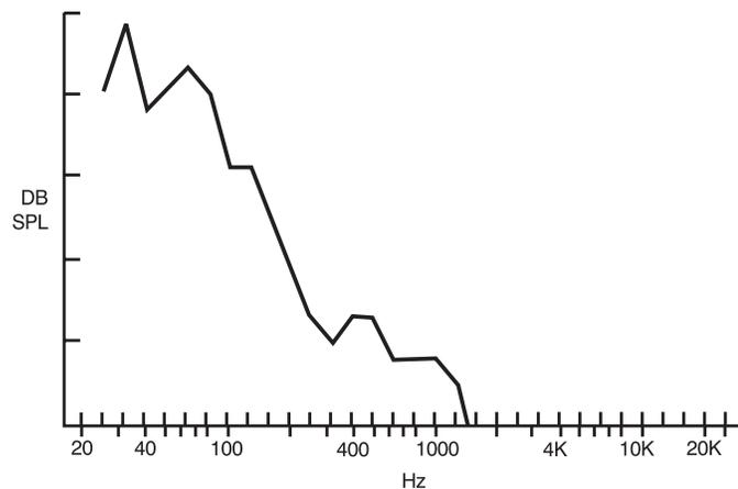
Fig. 1 The 1/3 octave response plot of road noise data for a typical car.
