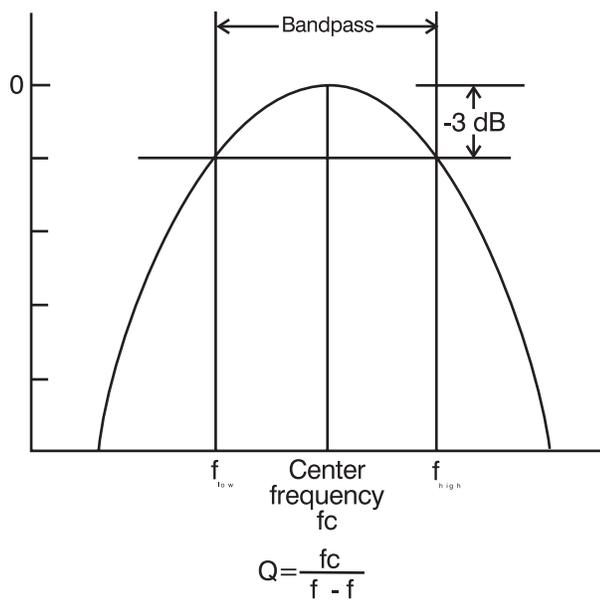
Figure 3. Bandwidth, Center Frequency and “Q”
