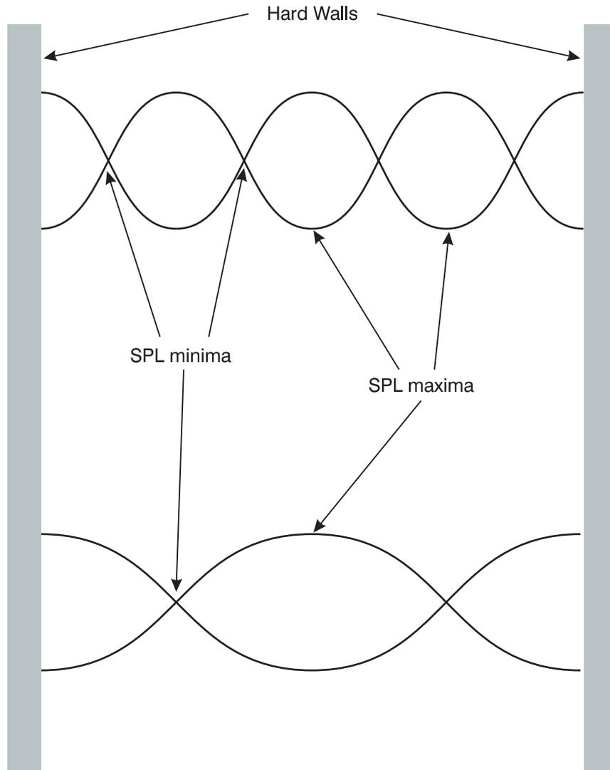
*Figure 4 - Standing waves between two parallel surfaces*
